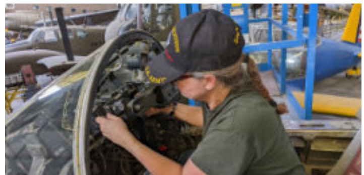
Deb installing the F-86 gunsight (K. Drewelow photo)
